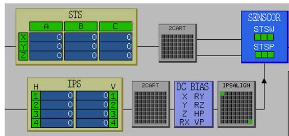
Figure 2: The MEDM Overview screen has been updated to show the new locations of the Bias and Alignment parts. The matrix values are not valid in this screen capture.
