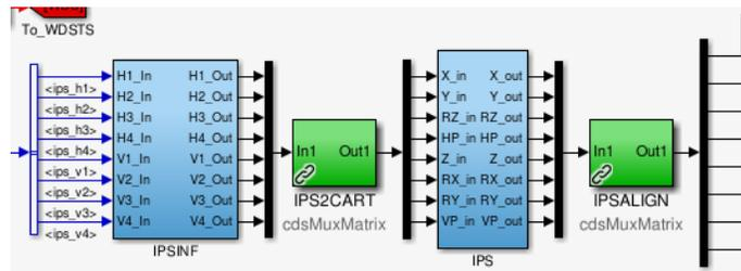
Figure 1: The location of the new cartesian basis bias block is just after the IPS2CART basis change. It is named IPS, which was chosen to give reasonable epic value names such as H1:HPI-HAM2\_IPS\_X\_LOCATIONMON. The new IPSALIGN matrix follows the monitoring to be sure the monitors are watching just the sensors, and not the user defined cross coupling.
