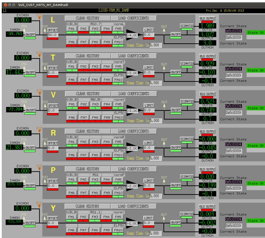
For a HLTS the damping gains in L,T,V,R,P,Y are [-5,-15,-15,-0.2,-0.01,-0.2].
