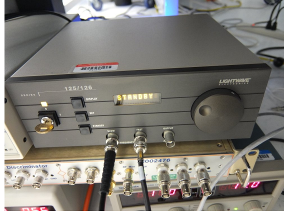
Figure 2: The Lightwave 126 power supply and controller.
