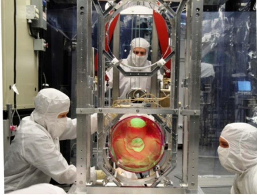
Figure 3: Advanced LIGO Large Optics Suspension, ( http://www.ligo.org/multimedia/gallery/opt.php ).
