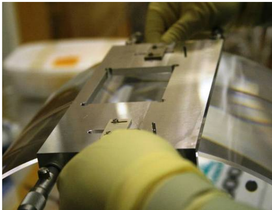
Placing bonding jig
