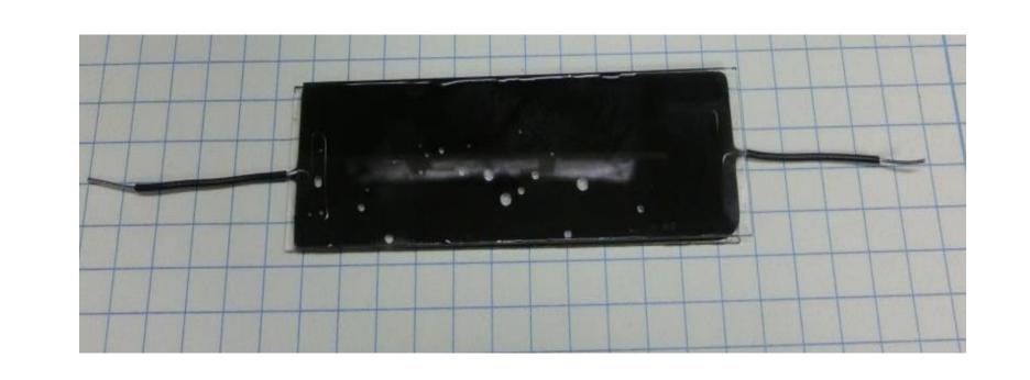
We are adding carbon to EpoTek in an attempt to make it conductive, and then re-test the new mixture for mechanical loss.
