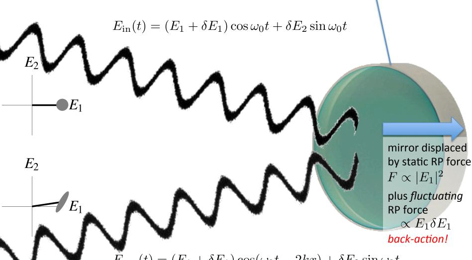
$$E_{\text{out}}(t) = (E_1 + \delta E_1) \cos(\omega_0 t - 2kx) + \delta E_2 \sin \omega_0 t$$
