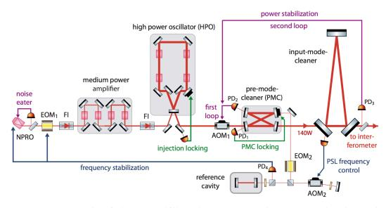
**Figure 4** Schematic of the pre-stabilized laser system. The Input Mode Cleaner is discussed in section 4.2. AOM: acousto-optic modulator; EOM: electro-optic modulator; FI: Faraday isolator; PD: photodetector.
