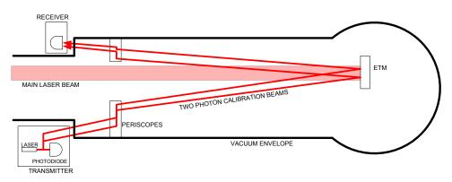
Figure 19 Schematic of the photon calibration system.
