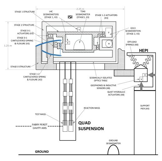
Figure 11 Seismic isolation for the test mass optic.
