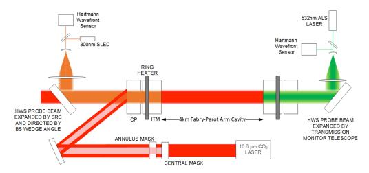
**Figure 13** Schematic layout of the Thermal Compensation System for the X-arm. A similar configuration is implemented on the Y-arm, with the SLED probe beam instead transmitting through the BS. Each of the masks can be independently flipped in or out of the beam path.
