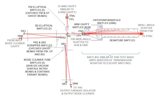
Figure 14 Locations of the primary scattered light baffles.
