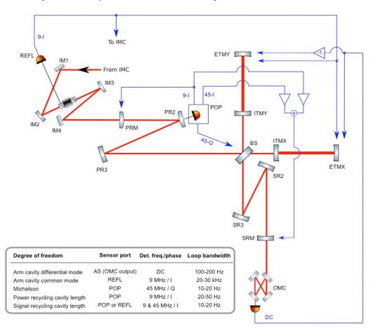
Figure 15 Length sensing and control scheme for Advanced LIGO. Though not shown, the Michelson signal is also fed back to the PRM and SRM, so that the BS actuation affects only the Michelson degree-of-freedom.
