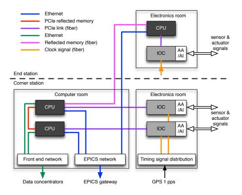
Figure 21 Schematic of the data acquisition architecture.
