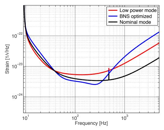
**Figure 3** Advanced LIGO strain noise spectrum for the modes defined in table 2, and for the nominal sensitivity shown in figure 2. The feature at 500 Hz is the (unresolved) fundamental vibrational mode of the test mass suspension fibres.
