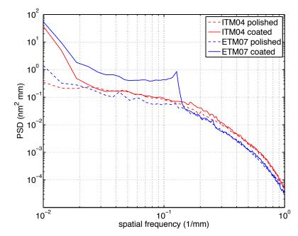
Figure 7 Power spectra of the surface maps, coated and un-coated, for the ITM and ETM used in one arm of the L1 interferometer.
