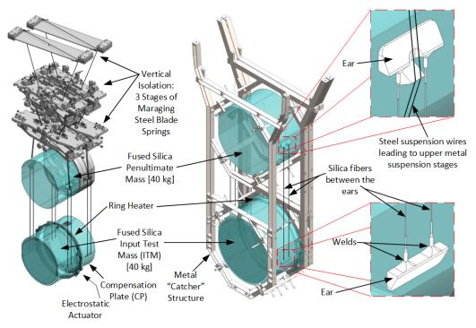
Figure 8 Quadruple pendulum suspension for the Input Test Mass (ITM) optic.
