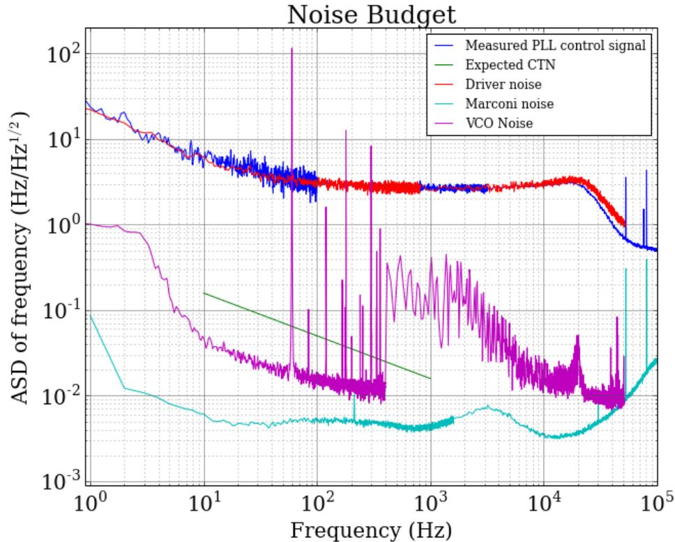
Fig 10. Noise budget of expected sources of noise in the setup
