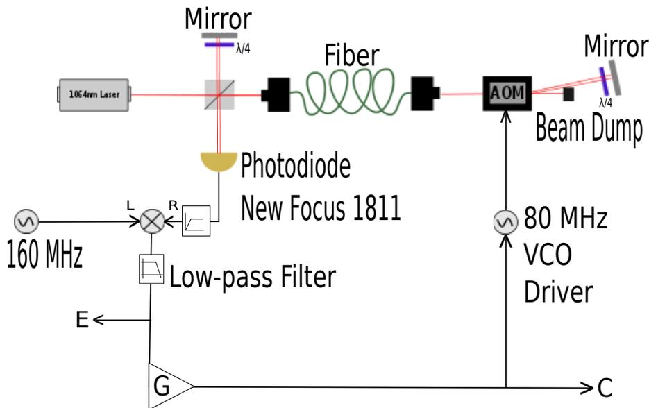
Fig 11. Setup of the 1 AOM fiber phase noise cancellation scheme
