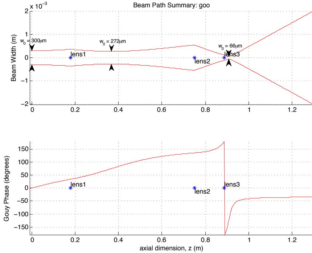
Fig 12. Mode-matching solutions for new lens placement yields a waist of 66 microns going into the fiber
