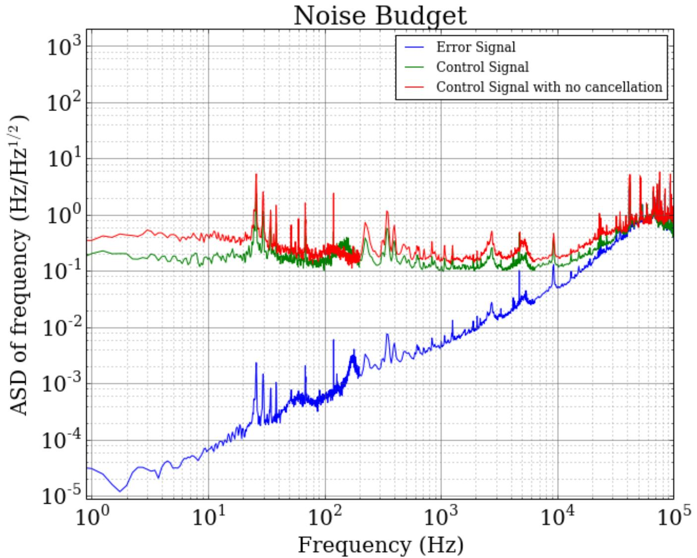
Fig 14. Measured PLL error signal and control signal with and without cancellation
