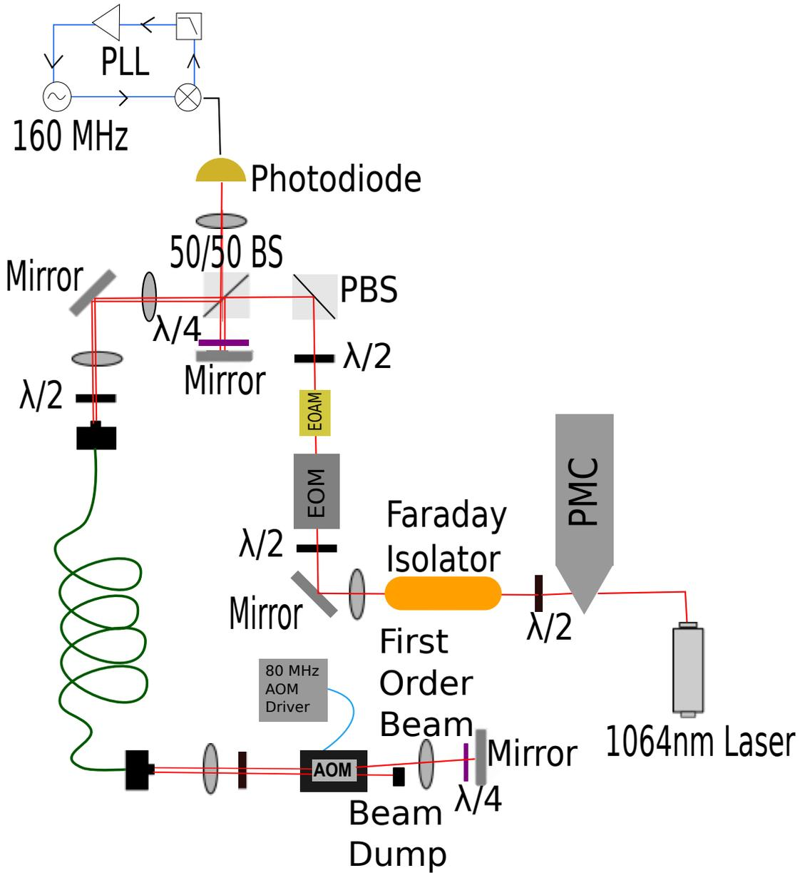
Fig 1. Table top set up for measuring fiber phase noise. The photodetector is connected to a phase-locked loop (PLL) to read the beat frequency, which gives fiber phase-noise information.
