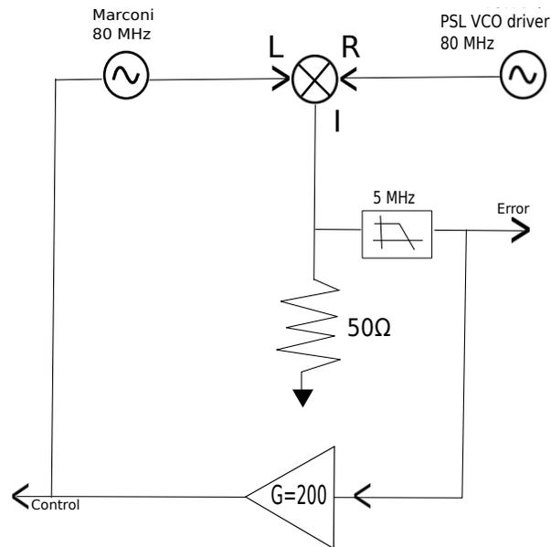
Fig 9. PLL setup for VCO driver noise
