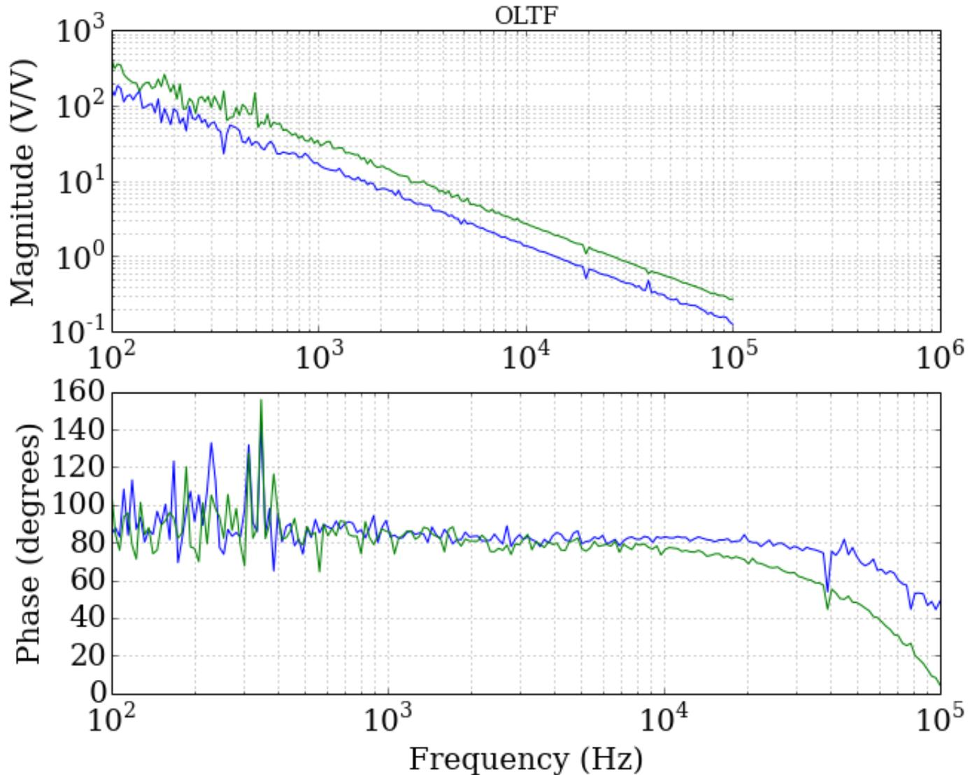
Fig 15. Measured transfer function with cancellation (green) and without cancellation (blue). The UGF when there is cancellation occurs at 27 kHz, the UGF when there is no cancellation occurs at 13 kHz
