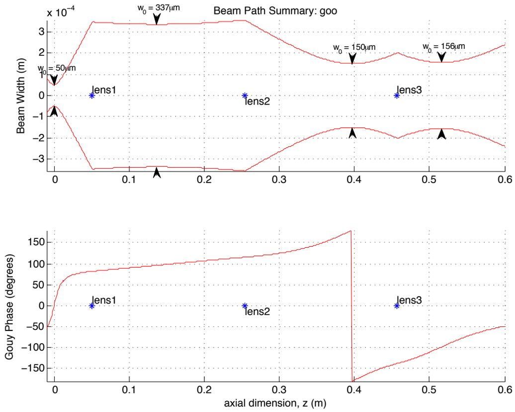
Fig 13. Mode-matching solutions for AOM double pass yields a waist of 150 microns going through the AOM and a waist of 156 microns at the mirror
