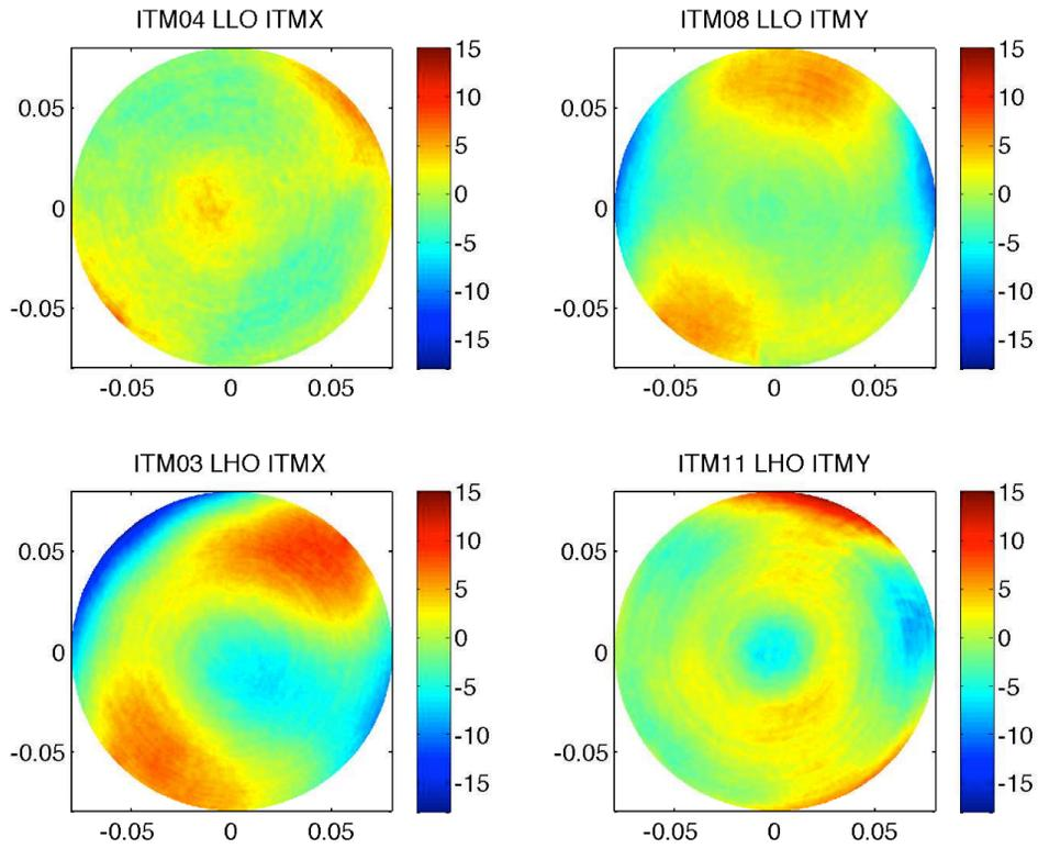
**Figure 2 SPTWE of L1 and H1 ITMs after subtracting tilt and power**
