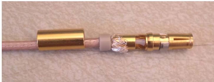
Figure 3, Accuglass 100909 contact assembly with RG-316 collet after final crimping
