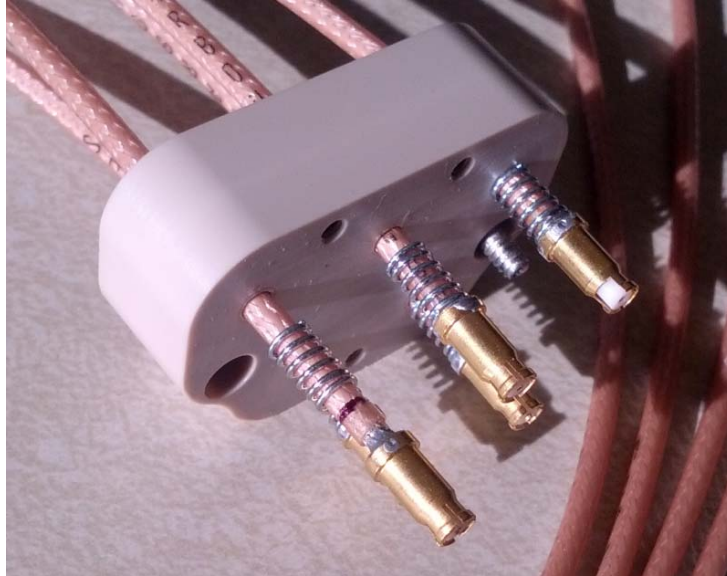
Figure 12, feedthrough taken apart, see little black band for indication of where to cut to maximize the remaining length
