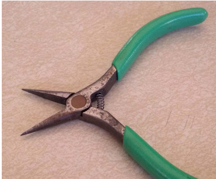
Figure 10, nice (rusty) pliers to grab and seat the socket inside the connector if needed
