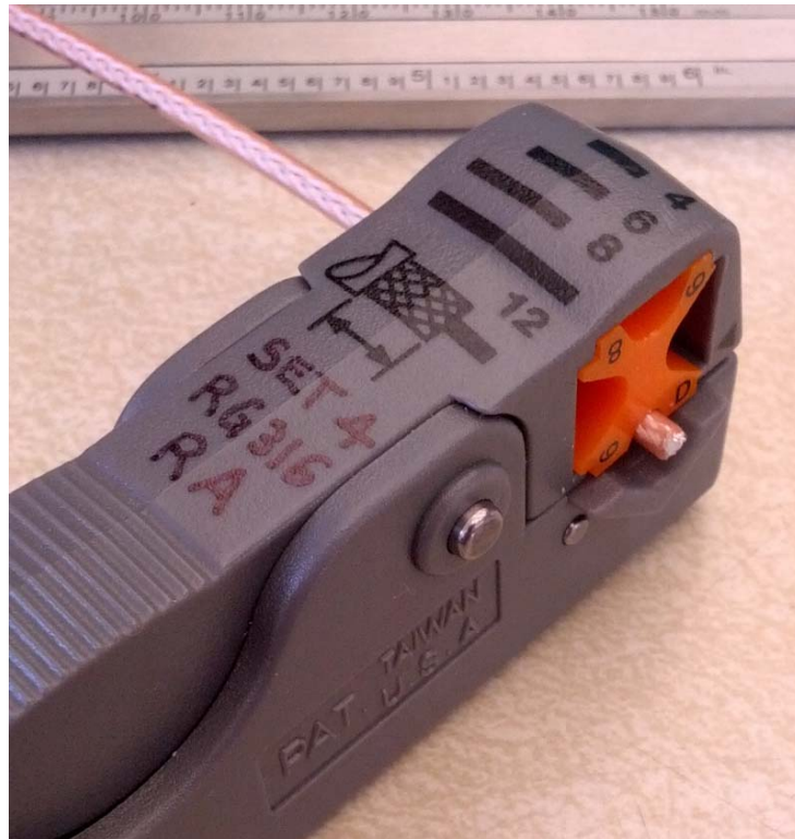
Figure 4, L-Comm RG-316 stripping tool. Note that the RG-316 protrudes flush with the right hand extreme of the stripper
