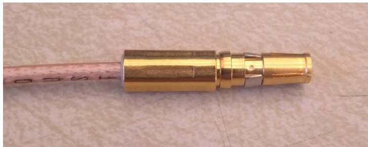
Figure 3, Accuglass 100909 contact assembly with RG-316 collet after final crimping
