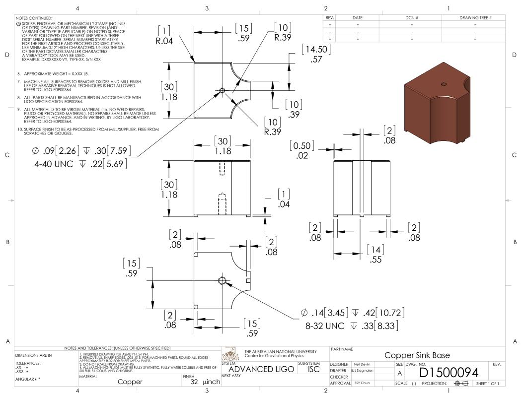
Copper Sink Base, PART PDM REV: , DRAWING PDM REV:
