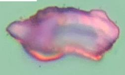
ETM14 Absorber Spot b) ~10 µm Located at (42,3) mm
