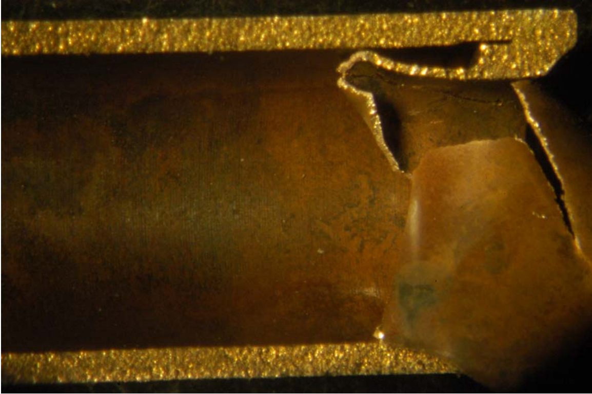
Inner surface of the support tube, after the flex tube has been peeled away on the right.
