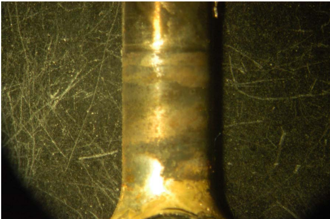
Detail of the press fit area on the flapper arm, after removing the flapper arm from the flex tube
