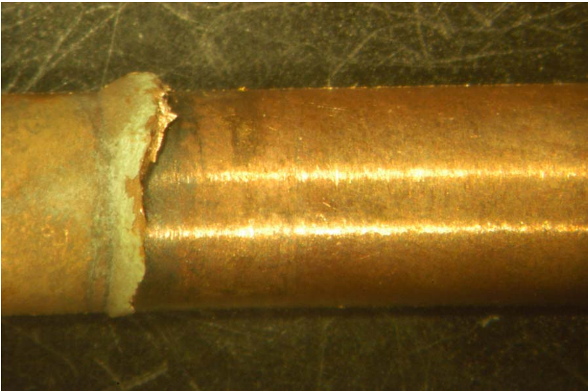
Press fit area on flapper arm, where flex tube was attached. It seems that some flux and/or braze material from the flapper arm/flapper tip joint crept up and partially brazed this joint as well.
