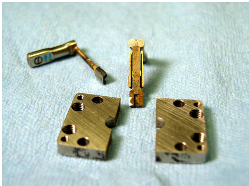
Figure 2. Flapper assembly sectioned by wire EDM.
