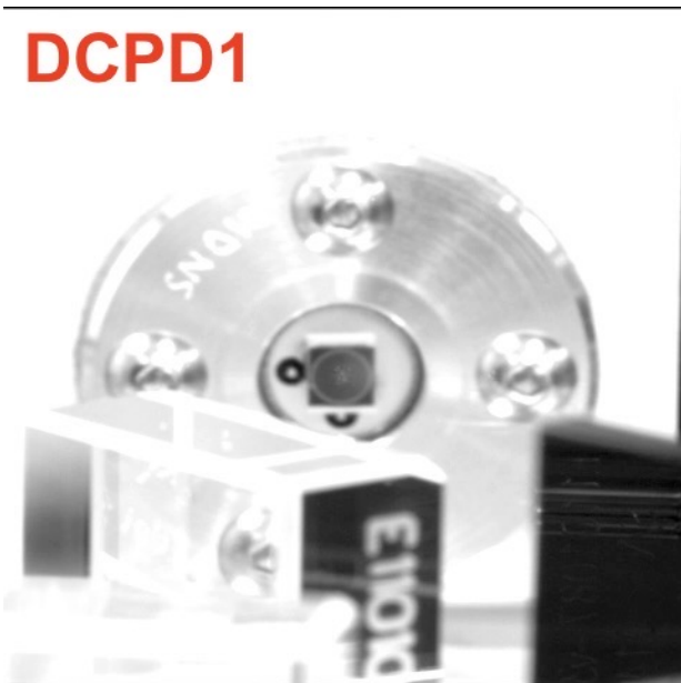
Figure 223: OMC(004): DCPD1 final spot position
