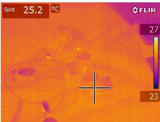
Figure 44: Thermal vision of the PZTs before the actuation.
