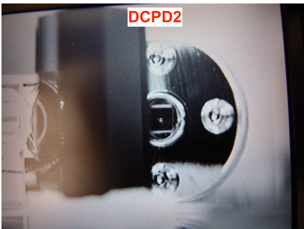
Figure 147: OMC(001): DCPD2 final spot position
