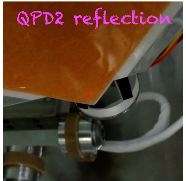
Figure 210: OMC(002R2): QPD2 reflection on the beam dump
