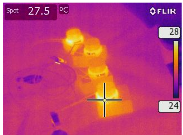
Figure 45: Thermal vision of the PZTs during the actuation.
