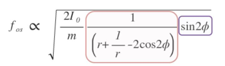
$I_0$ : laser power m: mass of the mirror *r*: reflectance of the mirror  $\varphi$ : detune phase
