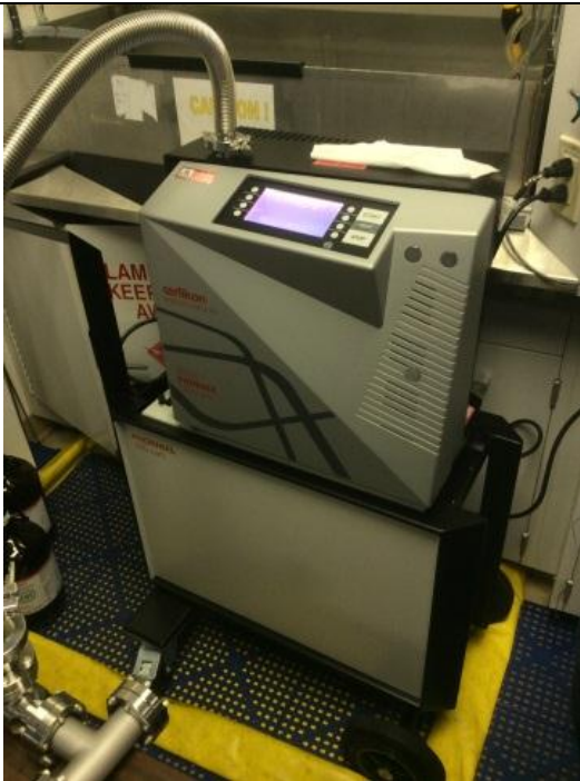
oerlikon Leybold Phoenix series, Model L300i Dry, Leak Detector
