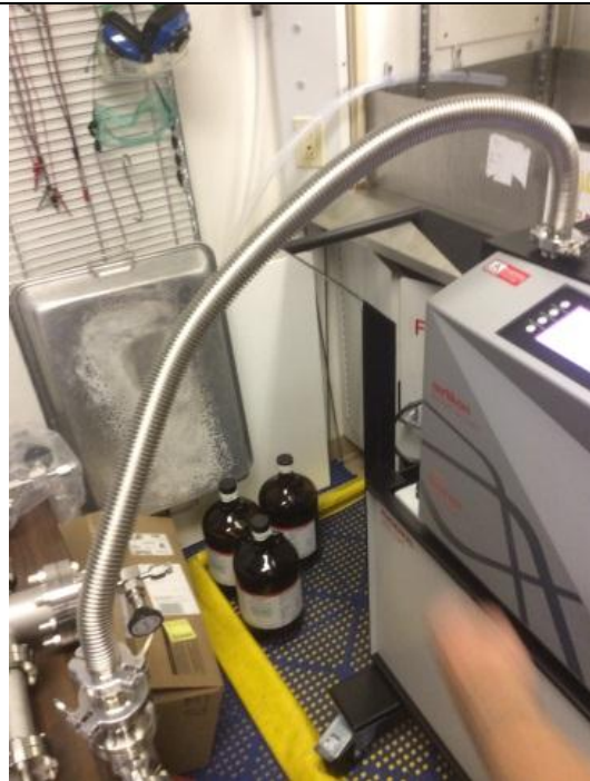
Pump fittings from DN25KF inlet port to device under test
