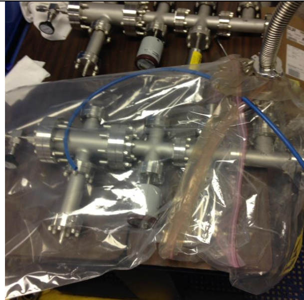
TMDS Ionizer Assembly in helium filled bag
