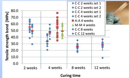
Figure 4.2 Tensile strength of sapphire-sapphire HCBs at room temperature for different curing times and C-C, A-A and M-M compared directly for 30 days curing.
