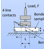
Figure 4.1 Schematic 4-point bend set-up to measure the tensile strength of the bond
