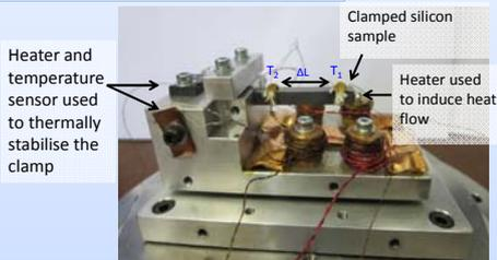
Figure 5.2 Silicon sample mounted in thermal conductivity set-up
