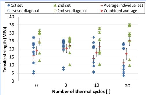
Figure 3.2 Tensile strength of silicon-silicon HCBs for different numbers of thermal cycles
