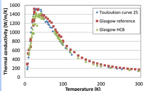
Figure 5.3 Thermal conductivity of both the reference sample and the bonded sample as a function of temperature compared to Curve 25 (Touloukian, 1977, Boron doped P-type silicon 6.2x 6.2mm silicon O-concentration  $7 \cdot 10^{17} / \text{cm}^3$ , resistivity  $3 \Omega \cdot \text{cm}$ ),
