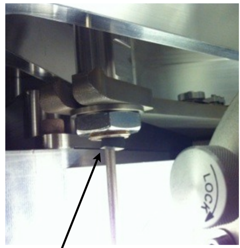
This piece of viton, from an iLIGO spring-seat, is normally used to damp the Tech Demo. This works very well, but is not appropriate for aLIGO because of uncertainty in drift, uncertainty in DC stiffness, and potential to fall out during an observing run.
