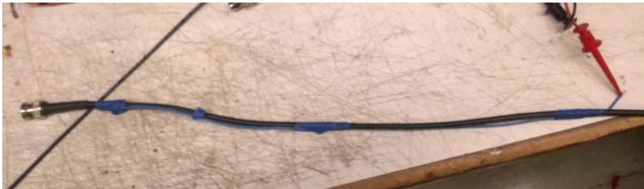
An RF signal generator was used to apply +13dBm signals to the far end (not shown in above photo) of the ~2m coaxial cable shown above. An RF spectrum analyzer was used to measure the amplitude of the signal induced in the sense wire (antenna).
