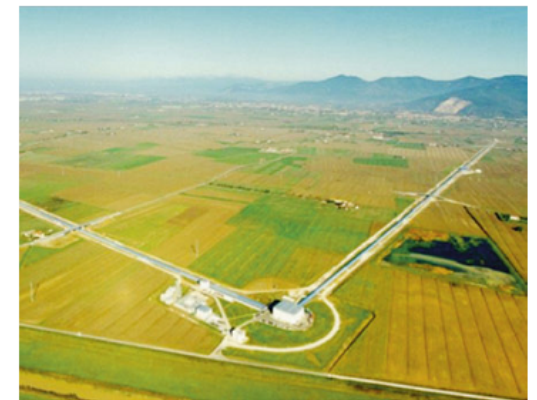
Fig. 1.2 – Virgo Detector, with 3 km arms, at Cascina, near Pisa
