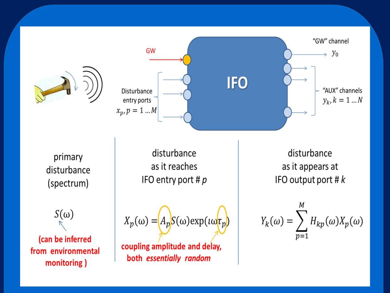
MIMO (Multiple-Input/Multiple-Output) model of interferometric GW detector. A transient disturbance reaches some "susceptible" entry ports, with random amplitudes and delays. The linear input-output relationships are described by linear transfer functions.
