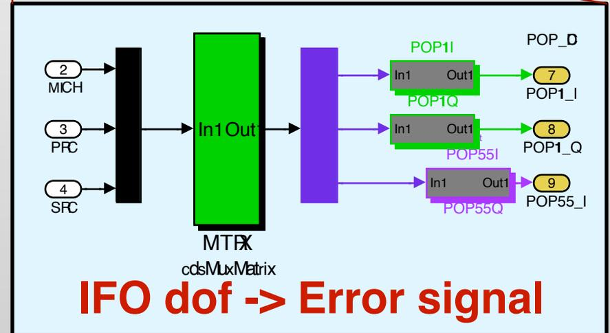
Formed by matrices and arrays(or matrices) of filter modules
