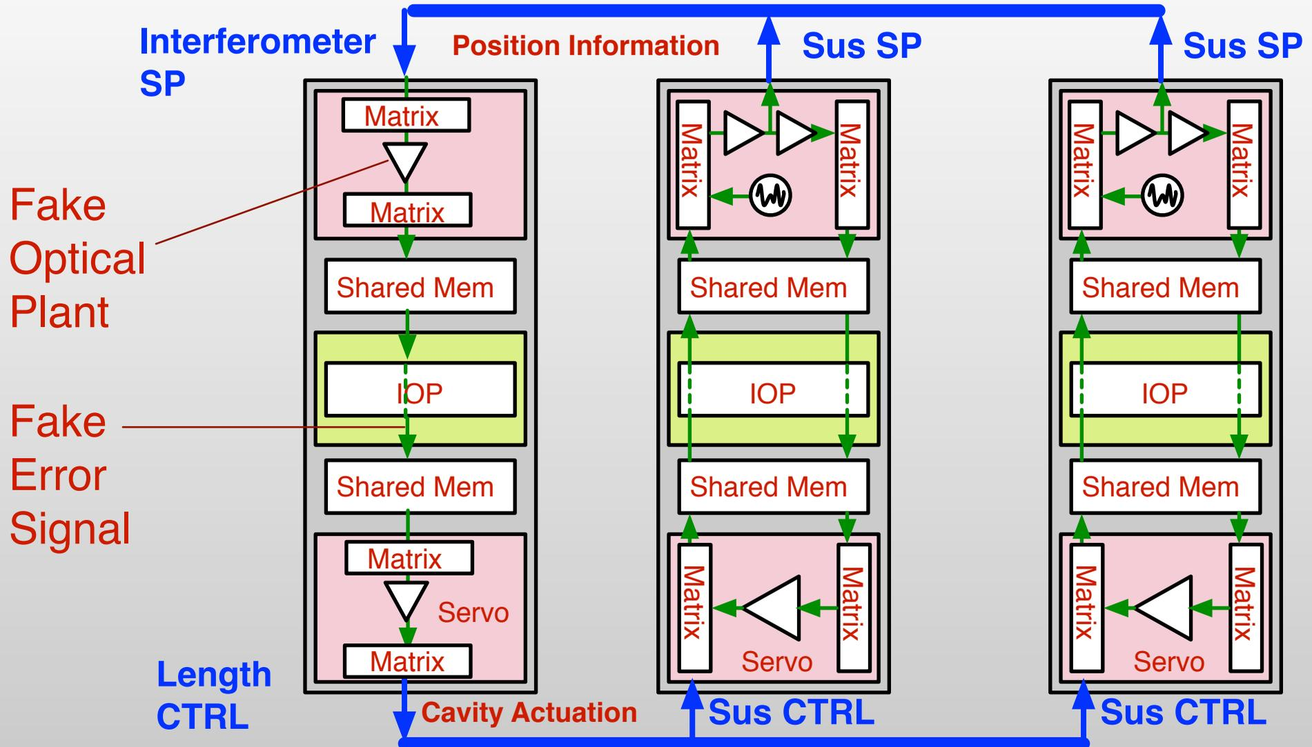
Formed by matrices and arrays(or matrices) of filter modules
