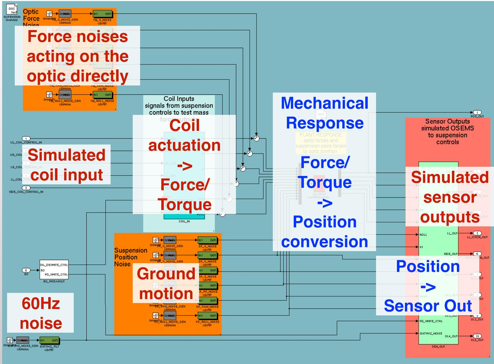
Formed by matrices and arrays(or matrices) of filter modules
