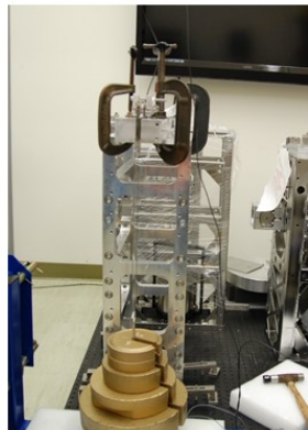
Pictures of overall set-up showing method of loading blade to its nominal flat position.
