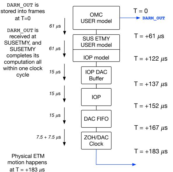
Actuation Function (From DARM\_CTRL\_WHITEN to Physical ETM Motion)
