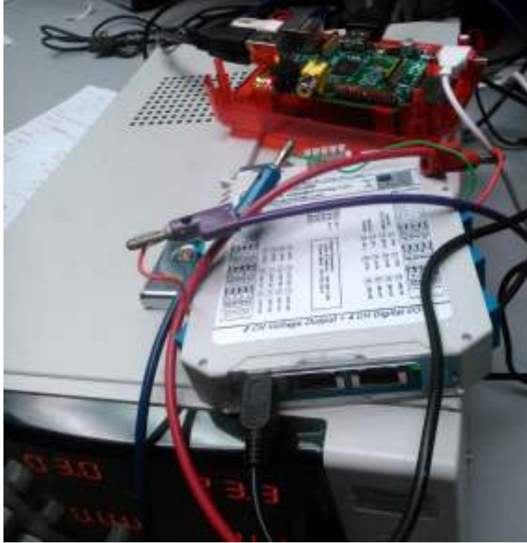
Figure 6: Photograph of DAQ Setup
