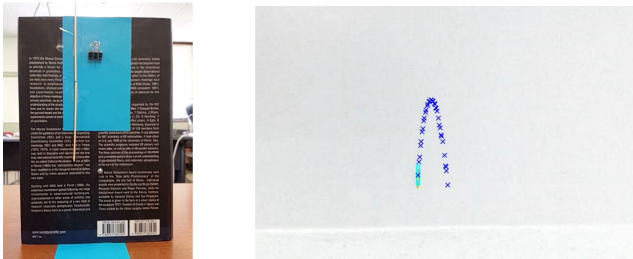
Figure 3: Early experimental setups for testing motion-tracking. The earlier experiment (right) demonstrates the binder clip and coffee stirrer release mechanisms. The later experiment (left) has a monochromatic background and demonstrates motion-tracking. The colors have been inverted for ease of viewing.
