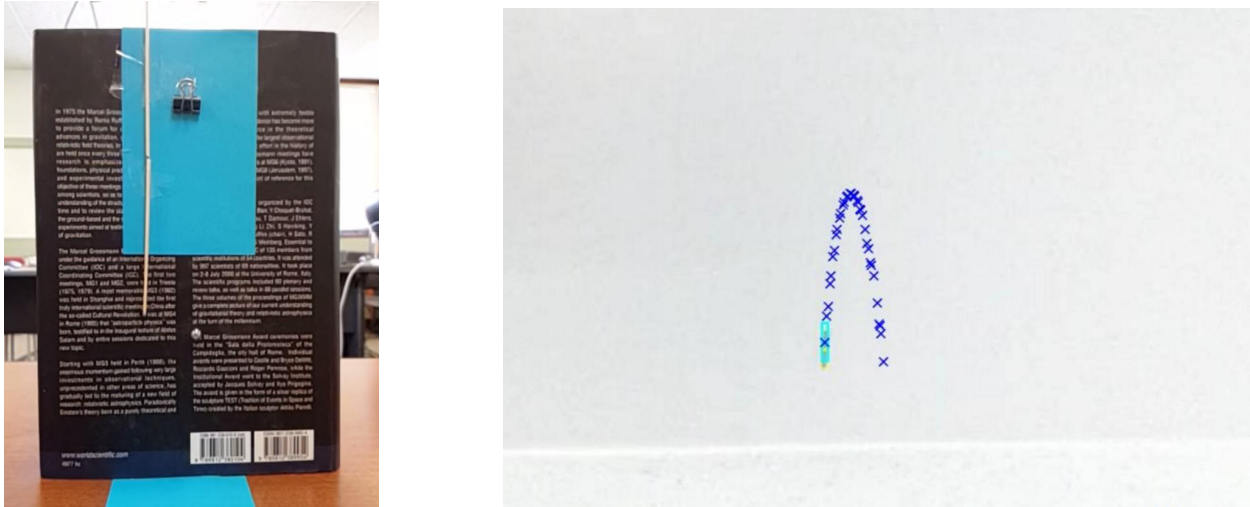
Figure 4: Early experimental setups for testing motion-tracking. A first iteration of the experiment (right) demonstrates the binder clip and coffee stirrer release mechanisms. A second iteration of the experiment (left) has a monochromatic background and demonstrates motion-tracking. The colors have been inverted for ease of viewing.
