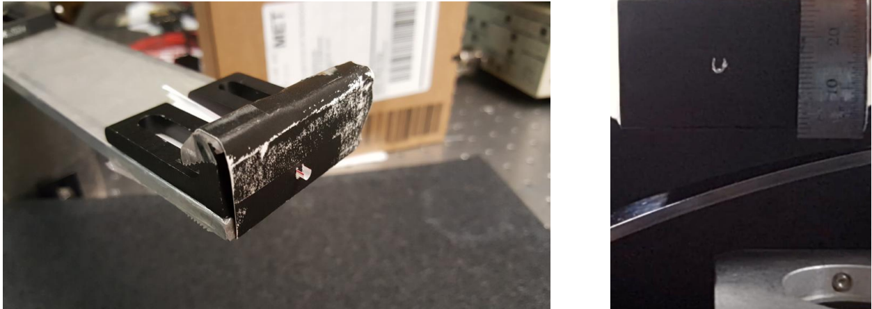
Figure 10: Two views of the final release mechanism for the ball drop experiment. Left: a top view of the mechanism consisting of half of a small straw poked through construction paper. A ball resting in the straw drops onto the blade when the straw is pulled through the paper. Right: a front view of the release mechanism, as seen by the camera recording experimental trials. One of the aluminum balls used is resting in the straw and a ruler is in the plane of the ball for calibration.
