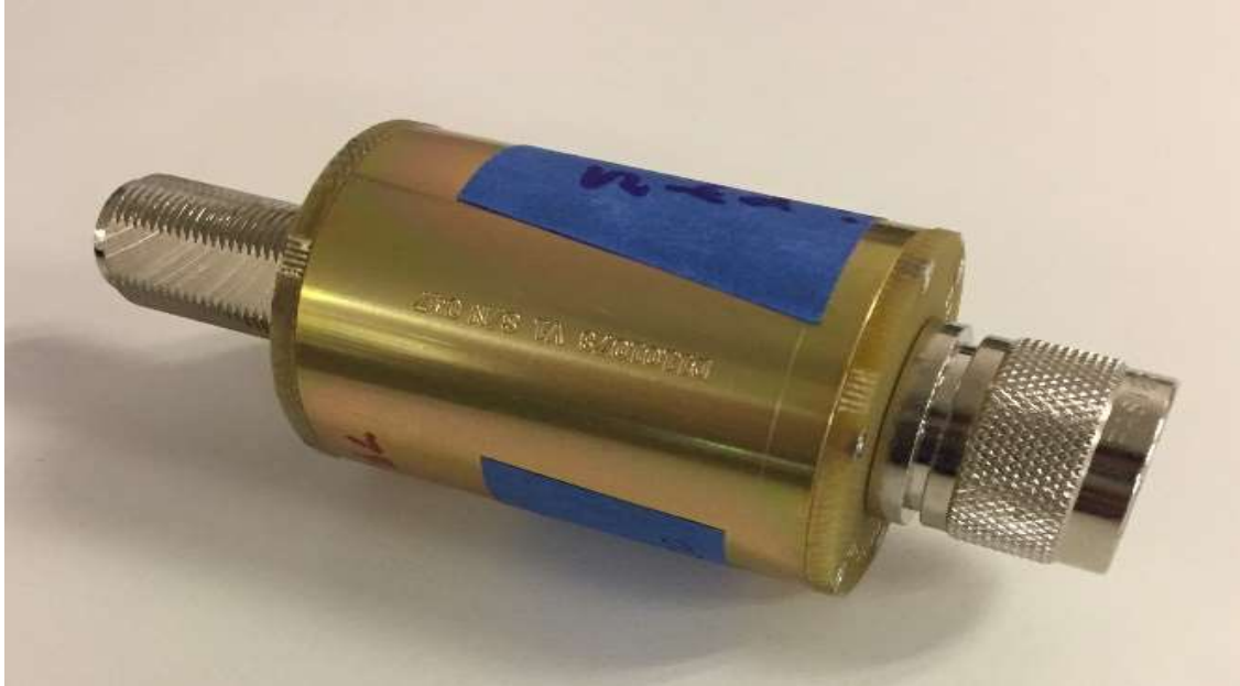
Figure 1a: DC ground isolation unit, or balun
