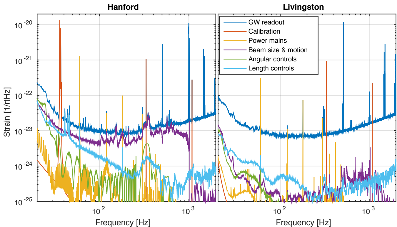
FIG. 1. Noise amplitude spectral density of the Advanced LIGO detectors (dark blue) with the left panel for Hanford and the right panel for Livingston. The other traces are the estimated contributions of the calibration lines (red), power line and harmonics (gold), beam jitter motion and beam size variations (purple), angular control noise (green), and the auxiliary length controls degree of freedom (light blue). These spectra are based on 1024s of data starting on 25 June 2017 at 08:00:00 UTC, at a time when both LIGO interferometers were operating and in an observation ready state.
