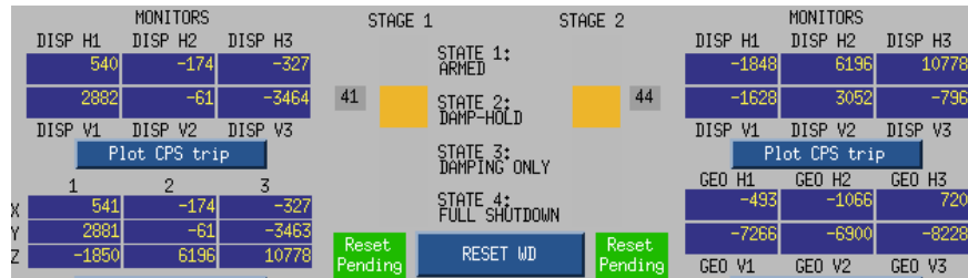
Figure 1: Detail of the updated watchdog screen - the system is damping, the countdown timer is running, and a reset is pending.
