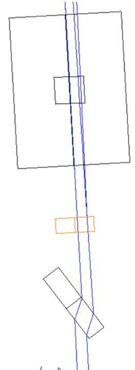
Output Brewster prism dumped by small baffles on OFI bench
