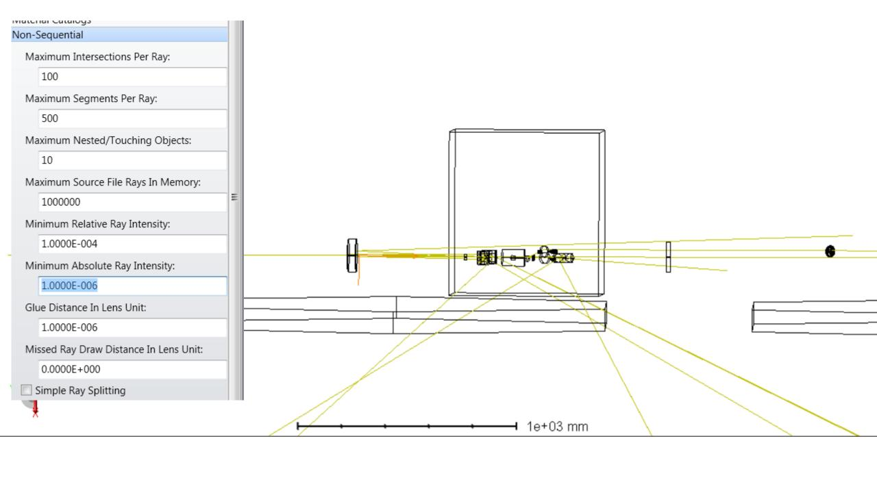
Input Wedge ghost beam dumped on SRM-AR baffle
