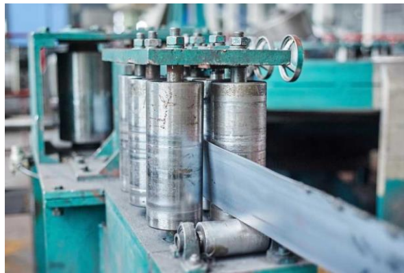
Figure 18. A commercial cold roller in a steel factory [25].
