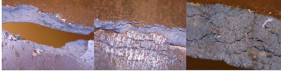
Figure 16. A mode 1 fracture in a maraging steel blade
