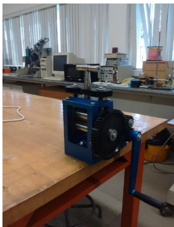
Figure 21. A small, table mounted hand-crank rolling machine
