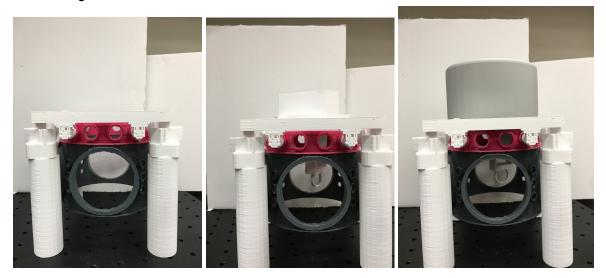
Here I have three pictures which represent the BSC Lower Shell Middle, Lower Shell Top, and the HEPI all glued and connected. In the second picture I have added the Quad Suspension for BS (or XY). The Quad Suspension does not need to be glued for the purpose of our hands-on model. Finally, in the last picture I have added the Top Hat which also does not need to be glued so one can look inside of the chamber by removing the hat.
