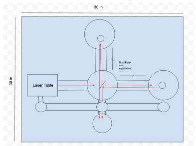
First the laser beam exits the laser table and arrives at the beam splitter. The beam splitter then splits the laser beam so that now there are two beams: one going straight towards the X axis mirror and one going perpendicular, towards the Y axis mirror. Both the X and Y mirrors then
