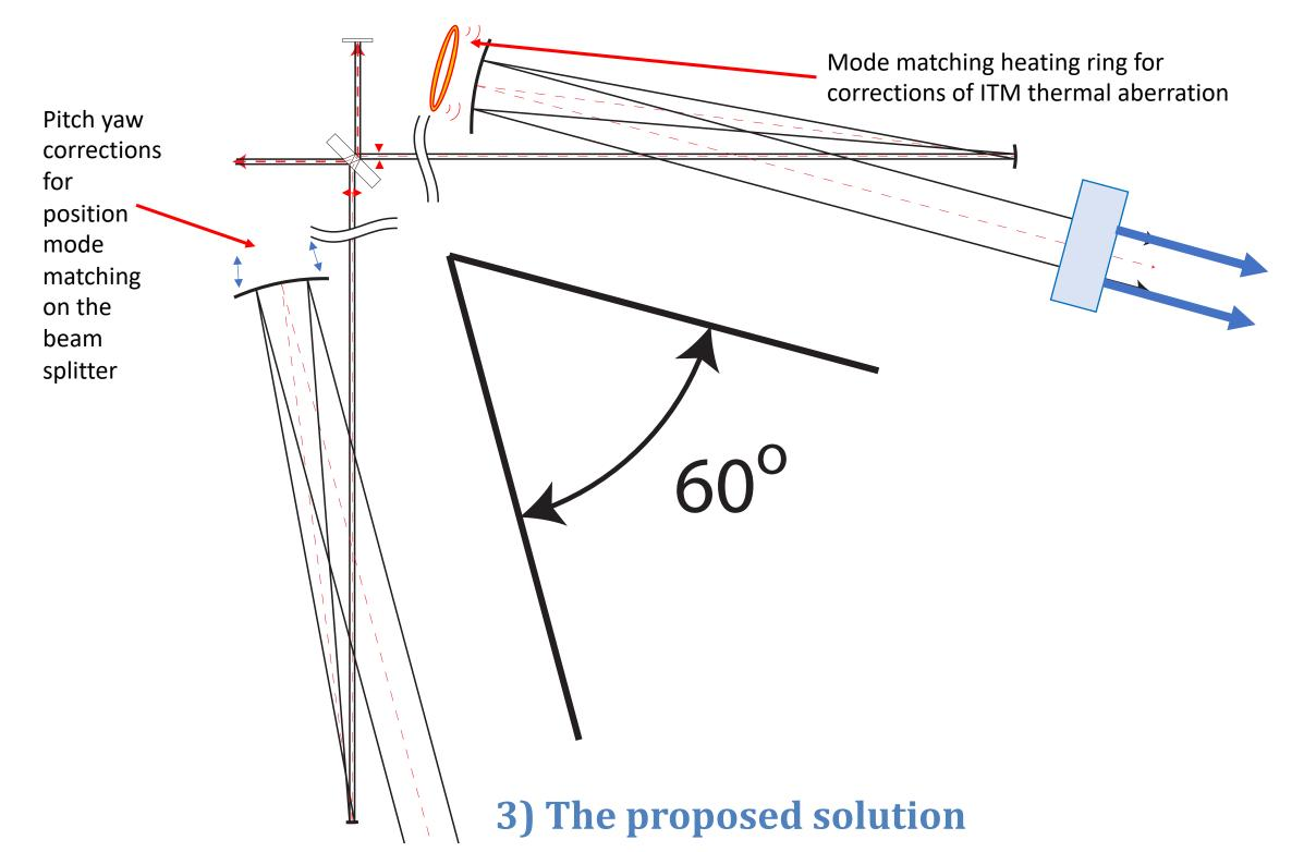
An arbitrary 203 mm beam diameter is chosen to illustrate the beam splitter size problem in the two configurations (actual beams would be much larger). A thickness vs. diameter ratio of 0.21 is chosen for minimal mechanical rigidity.
