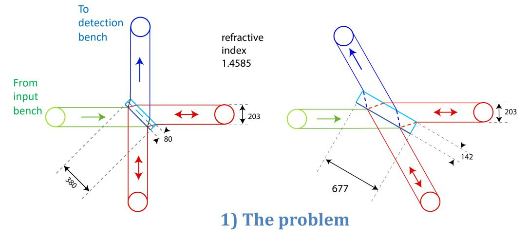
Beam splitter size comparison between the 60° and the 90° configuration.
