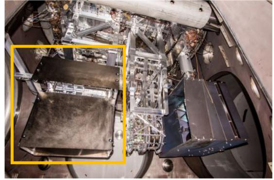
Installed shroud around TMSX (Transmission Monitor Suspension at X-end) and baffles on the photon calibrator periscope and on viewport nozzles. After the break the correlation with daytime noise is gone. See alog entry here.
