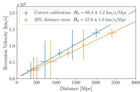
FIG. 4. A toy model of how the estimate of the Hubble constant,  $H_0$ , may be skewed by 20% systematic error in detector network calibration (20% is an exaggerated level of systematic error to demonstrate the effect). Error bars indicate individual events and their uncertainty (with presumed systematic error). The gold solid line indicates the resulting (biased) estimate of  $H_0$ . The blue line indicates an example “true” value of  $H_0$ .
