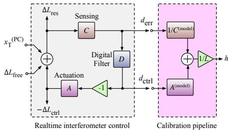
FIG. 1. Simplified diagram of the differential arm length control loop of the detectors. The digital error,  $d_{err}$ , and control,  $d_{ctrl}$ , signals are converted to an estimate of the strain on the detector in the absence of the control system,  $h = \Delta L_{free}/L$ . The model for such conversion is referenced to the photon calibrator system, which causes displacement,  $x_{PC}$ , equivalent to  $\Delta L_{free}$
