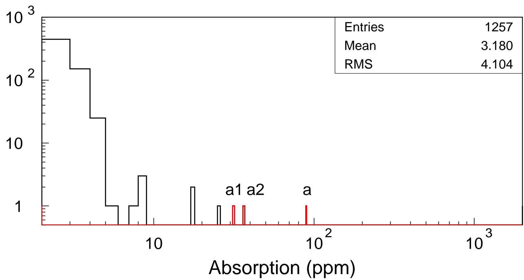
SN0932, point a, removed by laser ablation.
