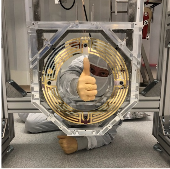
Figure 4-2: The installed end reaction mass (ERM) showing the installed electrostatic drive (ESD) pattern. Prior to O3 the original end reaction masses (ERMs) were replaced with annular ERMs, in which the center section was removed to reduce the effects of squeezed film damping. Photo credit: Gary Traylor and Danny Sellers
