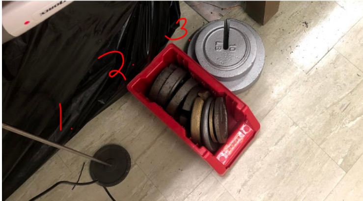
Figure 8: Weights used in second setup: 1. the 1 lb stand used, 2. is the standard weights, 3 the heavier weights, 10 lbs+.
