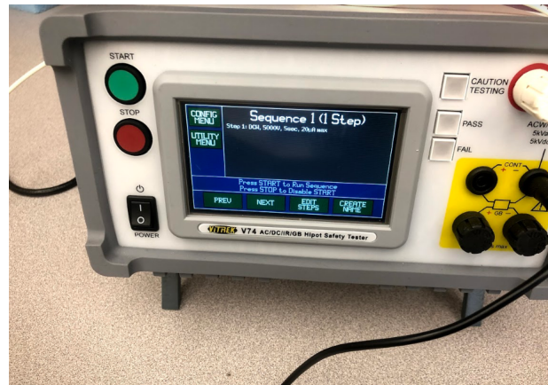
Figure 2: Hipot Tester used, Vitrek V74 Hipot Safety Tester. Notably, the maximum voltage able to be applied is 5000V.
