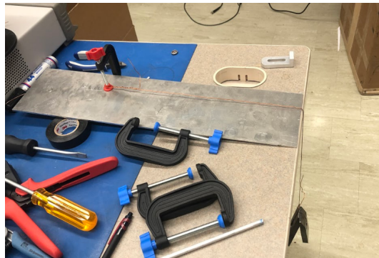
Figure 4: Apparatus Diagram for First Experimental Setup. The wire is wrapped around the C-clamp clamped to a metal sheet. It then hangs off the sharp edge.
