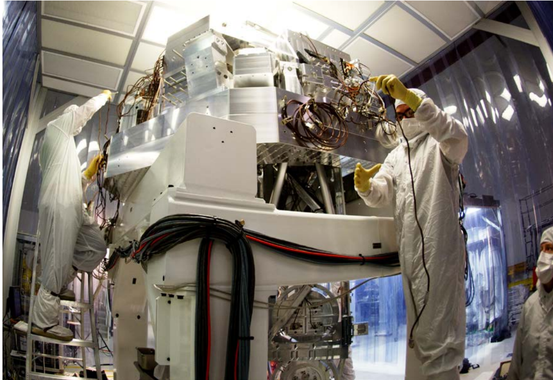
2-stage internal seismic isolation (ISI) system (test mass optics, large chambers)
