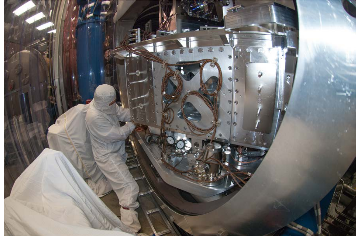
1-stage internal seismic isolation (ISI) system (smaller chambers, input & output optics)
