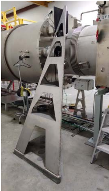
Optical Lever Transmitter & Receiver for the Input Test Mass (ITM)
