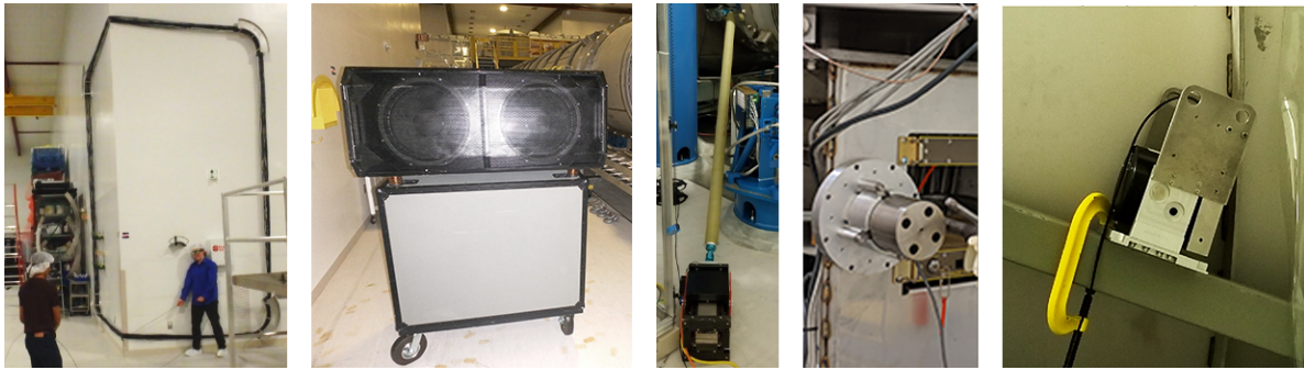
Figure 6. Injection equipment photos. From left to right: wall-mounted magnetic field injection coil; 14-in. speakers; APS 113 shaker connected to the door of a vacuum chamber by a rigid fiberglass rod; modified Piezosystem shaker clamped to an electronics rack; modified B&K shaker clamped to a beam tube support.
