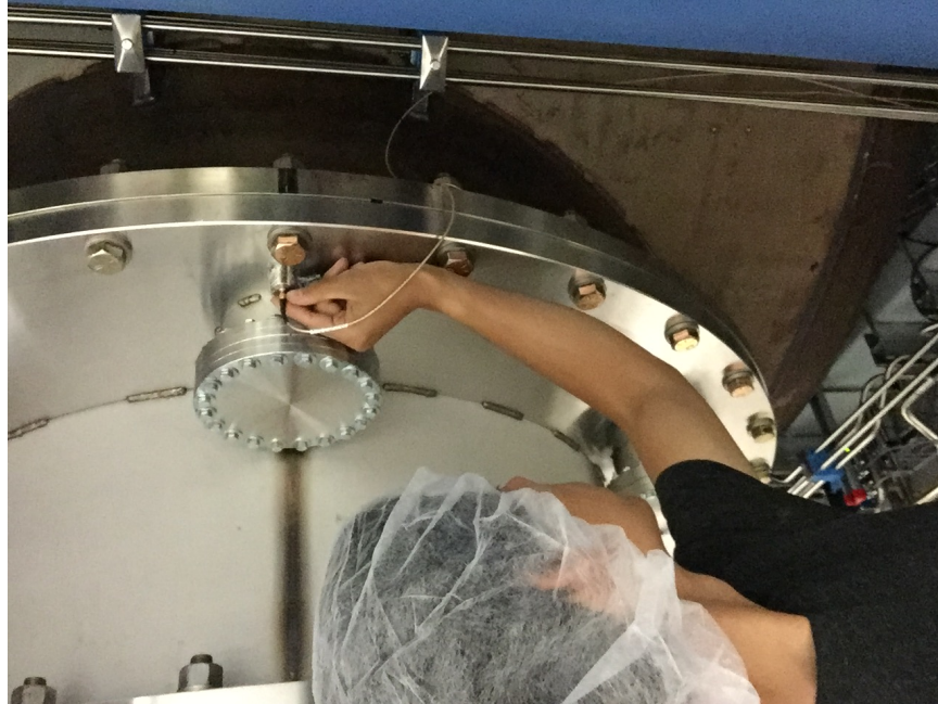
FIGURE 5.2. The author installing an accelerometer on a vacuum chamber at LIGO-Hanford.
