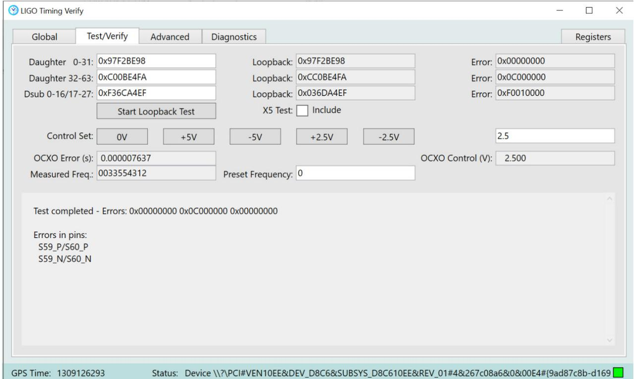
Connect an OCXO, for example T0900279, to SMA input J5 on the rear side of the board. Check the measured frequency.
