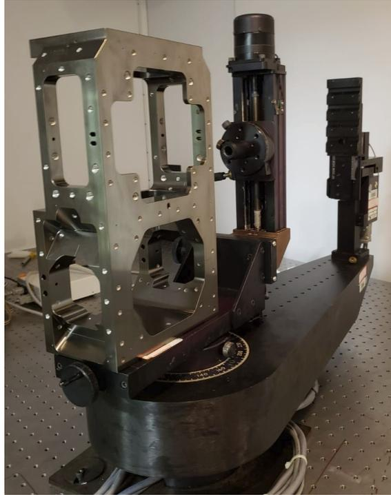
Figure 3. HDS structure on Scatterometer. The first set of measurements were taken with this configuration. For future measurements, the laser was pointed at another surface on the structure.
