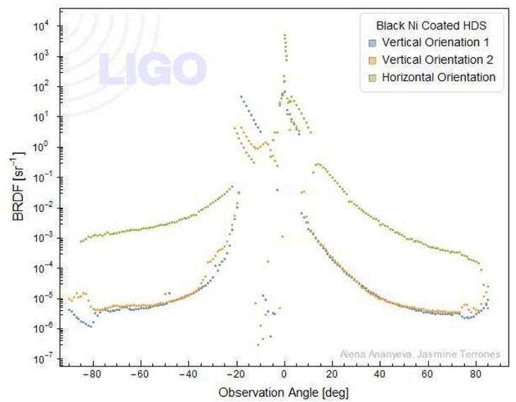
The vertical orientation plots both have very strange dips near the top of their curve. This is likely due to some calibration error on the scatterometer. The HDS structure will be measured again in the vertical orientation to obtain better data
