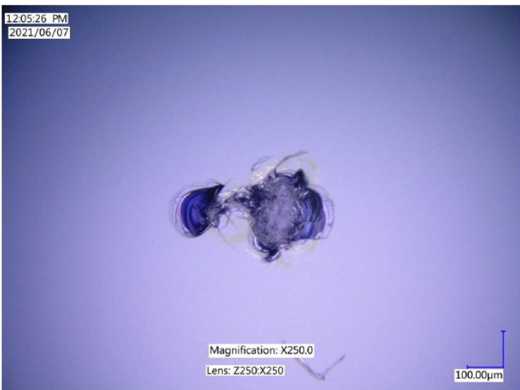
SN0668, M2, laser burned mark (on black ink)
