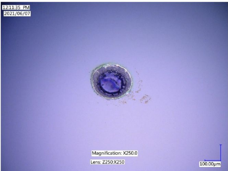
SN0668, M2, laser burned mark (on black ink)
