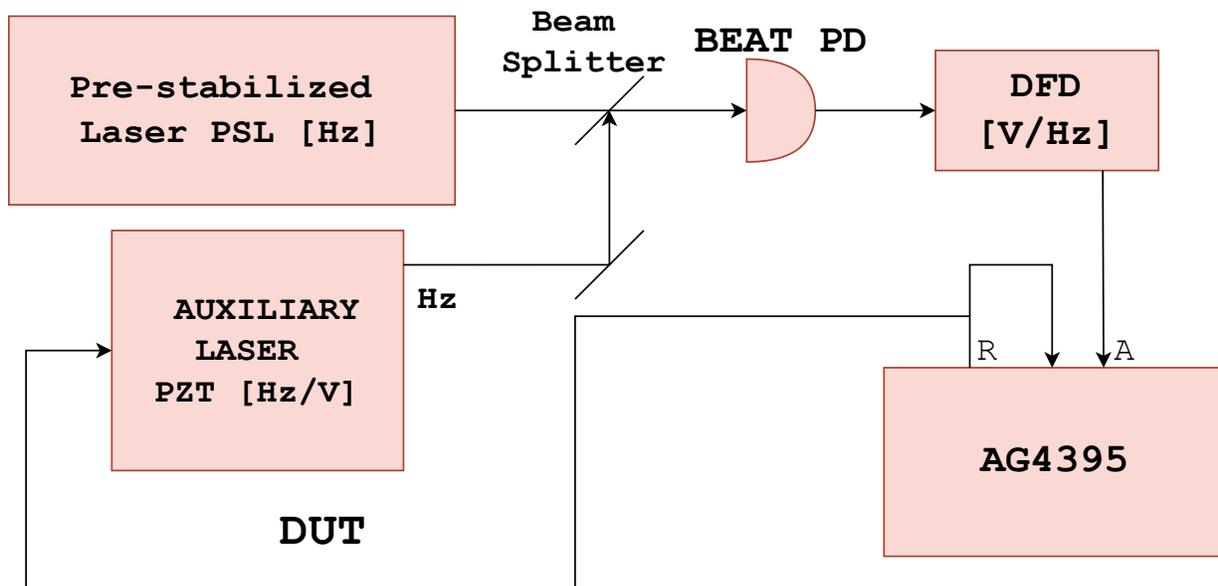
Figure 2: Experimental Setup using the Delay Line Frequency Discriminator [4]
