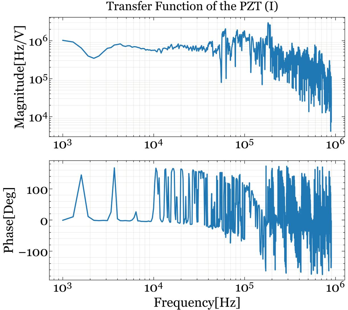
Figure 4: PZT Transfer Function as measured by the DFD
