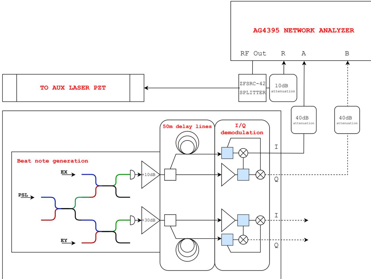
Figure 3: Detailed Schematic of Delay Line Frequency Discriminator [3]
