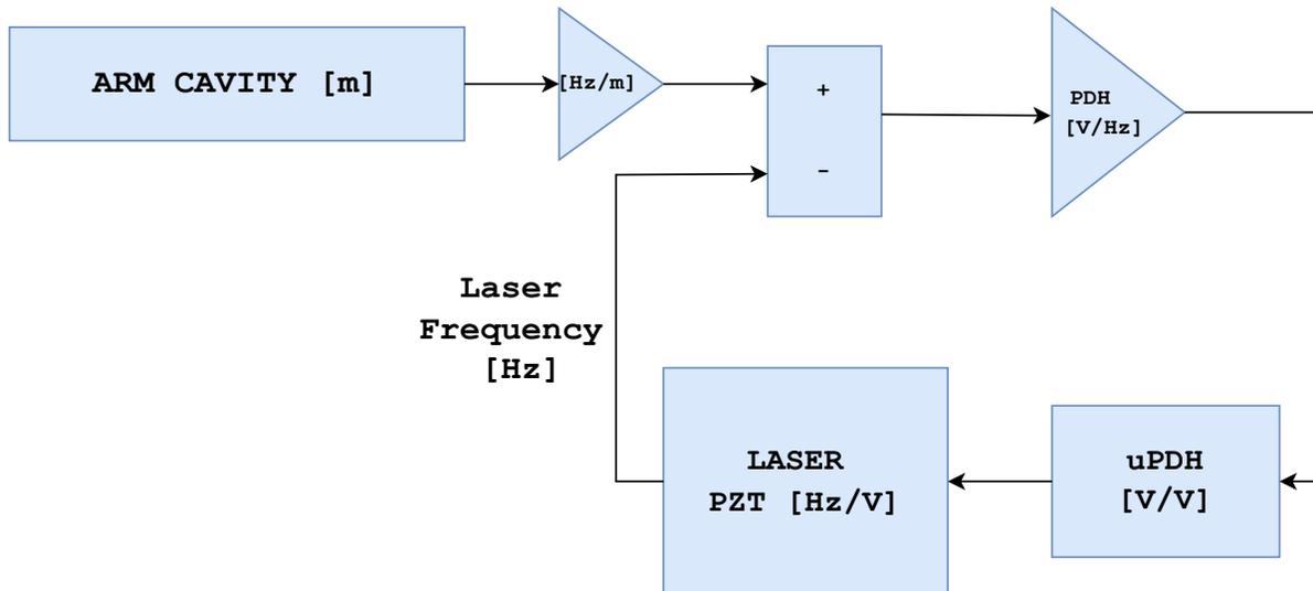
Figure 1: Thematic diagram of the AUX Loop
