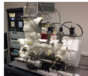
VORTEX: Table top experiment to investigate material outgassing.
