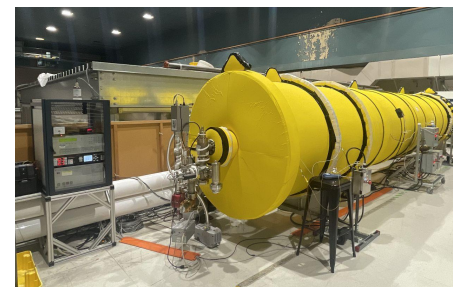
LTREX: 7.5 m long, 1.2 m diameter, 3 mm wall thick residual section of iLIGO beamtube, matches BT surface properties, used to explore emergency venting/recovery protocols at LIGO.
