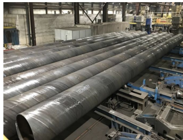
Gas pipe mill: Mills capable of large order sizes and established QA system in place for fuel gas pipeline safety (US DOT).
