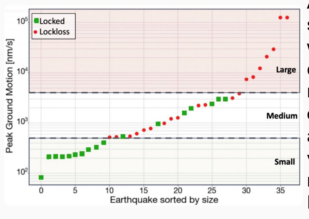
An early warning strategy, together with control changes can be used to mitigate the impact Medium of earthquakes with a peak local ground velocity of 500-2000 nm/s in the sub 0.1 Hz band.
