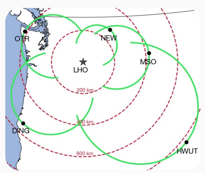
The solid lines represent virtual locations of the stations events for incoming from different azimuths. They form a protective 'fence' around the detectors.
